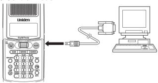
To connect the Scanner to a PC, plug the scanner end of the supplied RS232C cable into the remote port which is on the side of the scanner. Plug the other end of the cable into your PC's serial port.
