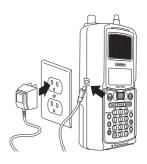
**Note:** Disconnect the AC Adapter/Charger from the unit when charging is complete.
