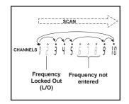
4. When a transmission is received, the LCD back light comes on for five seconds and the scanner stops on that channel, provided that you have selected the Auto Light feature. When the transmission ends, scanning resumes automatically.
