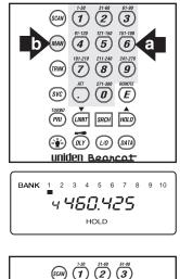
Press and hold (PR) /TURBO for two seconds to designate this channel as your new Priority Channel.
