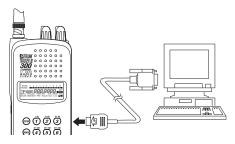
Plug the smaller end of the supplied RS232C cable into the remote port which is on the right side of the scanner. Plug the other end of the cable (DB-9 serial connector) into a personal computer's serial port. A few PC's may require an adapter, most will not. You may need a DB-9 to DB-25 null modem adapter, available at most computer stores. Of course, make sure your PC is turned on.
