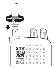
Attach the flexible antenna to the **BNC** connector.
