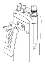
Do not tighten the screws too tight. You can damage the case or clip.
