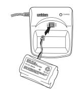
Place the battery in the charger, and plug the AC Adapter into a wall outlet.
