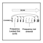
4. When a transmission is received, the Scanner stops on that channel. When the transmission ends, scanning resumes automatically.
