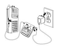
2. When charging is complete, disconnect the CRX120 from your scanner, then unplug the AC Adapter/Charger from the CRX120.
