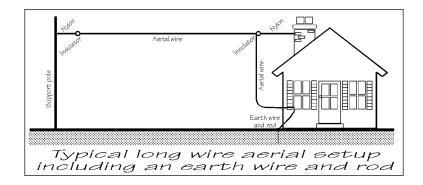
**Magnetic balun** long wire aerials are becoming very popular as they allow coaxial cable to be used as the down-lead from the wire aerial into the receiver. The balun transforms the impedance to a low level suitable for 50 OHM coaxial cable. In this instance the path of feeder is unimportant and chances of noise entering the aerial system reduced. The 50 OHM BNC aerial input of the AR3030 should be used and selected accordingly.
