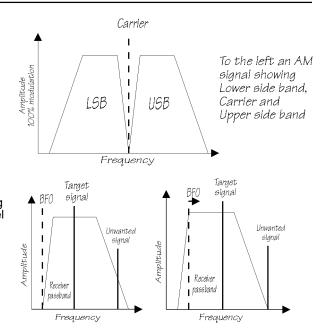
Above left: SSB true carrier re-insertion showing an unwanted signal in the passband. Above right: the receiver has been tuned downward
