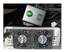
Turn off your Kenwood<sup>TM</sup> transceiver. Plug the 6 pin connector into the tuner jack on the back of your Kenwood<sup>TM</sup> transceiver. When the transceiver is powered-up, a signal from the k-Box Controller tells the transceiver that an antenna tuner is connected.
