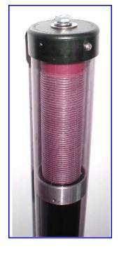
or decrease inductance until a sharp dip occurs. Adjust for lowest reading by moving the control switch back and forth. You are now tuned to 7200kHz.
