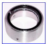
Over time (and especially in salt water environments) you may find some aluminum oxide build-up under the spring in the 'decoupler.' Simply remove the spring and clean the aluminum surface with steel wool. Put a *small* amount of an antioxidant (such as NO-OX) in the groove before replacing the contact spring. A 'Q-Tip' cotton applicator works well for this purpose.
