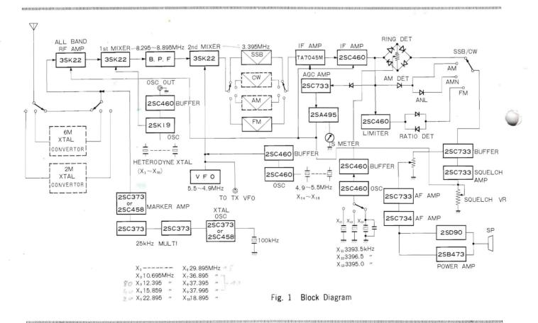
is injected through gate 2. Thus, 1st mixer Q2 comprising FET 3SK22 heterodynes its input signal with 1st local oscillator output to deliver the 1st IF signal ranging from 8.295 to 8.895 MHz.
