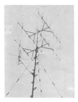
Photo 3 An Example of Antenna (For VHF)
