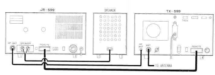
Fig. 6 Connection Diagram for a Combination of models JR-599 and TX-599
