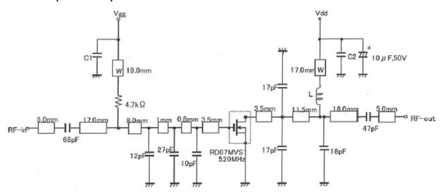
Note: Board material-PTFE substrate, Micro strip line width=2.2mm/50Ω, εr=2.7, t=0.8mm
