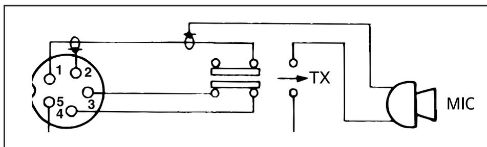
Fig. 1. Cobra 2010 GTL WX microphone schematic.
