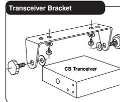
A universal mounting bracket is supplied along with self tapping screws and star washers. The transceiver is held in the universal mounting bracket by two thumb screws, permitting adjustment at the most convenient angle.
