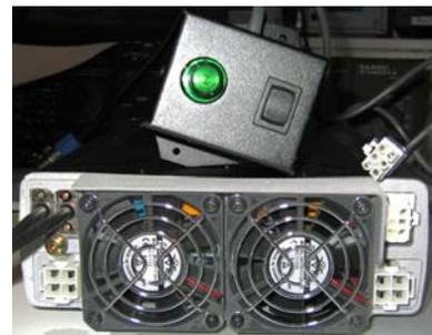
Turn off your Kenwood™ transceiver. Plug the 6 pin connector into the tuner jack on the back of your Kenwood™ transceiver. When the transceiver is powered-up, a signal from the k-Box Controller tells the transceiver that an antenna tuner is connected.
