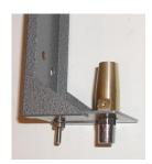
The matching coil is not needed. With radials attached to the screw on the mounting bracket, the antenna will tune to resonance with an impedance close to 50 ohms.
