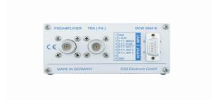
The remote powering coupler DCW 2004 B allows a comfortable remote coupling of our SUPER-AMP preamplifiers via the coaxial cable as well as for delayed switching of HF-linear amplifiers.
