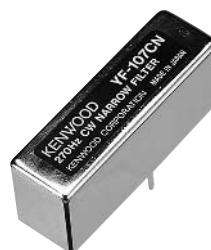
YF-107CN (270Hz CW Narrow Filter)
