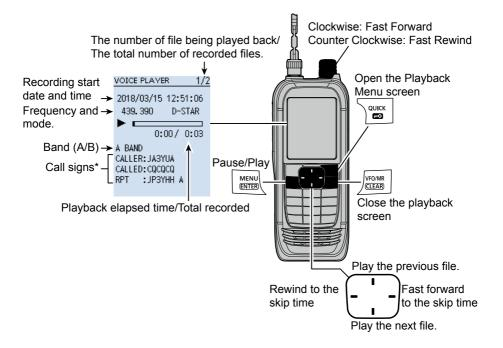
\*When the receive mode is D-STAR, the received signal's call sign is displayed.
