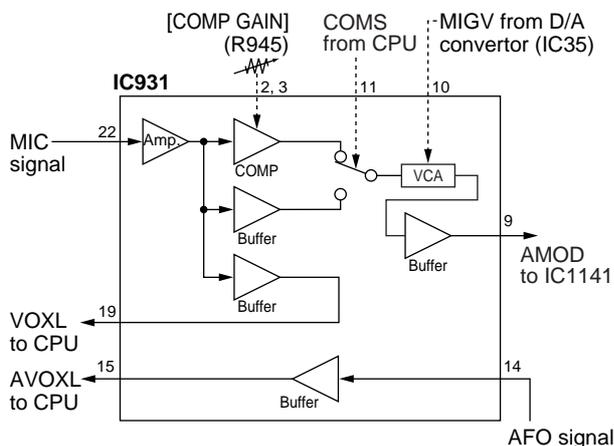
Audio signals from the front or rear panel [MIC] connector enter the microphone amplifier IC (IC931, pin 22) and are then amplified at the microphone amplifier or speech compressor section. Compression level is adjusted with the [COMP GAIN] control (R945).
