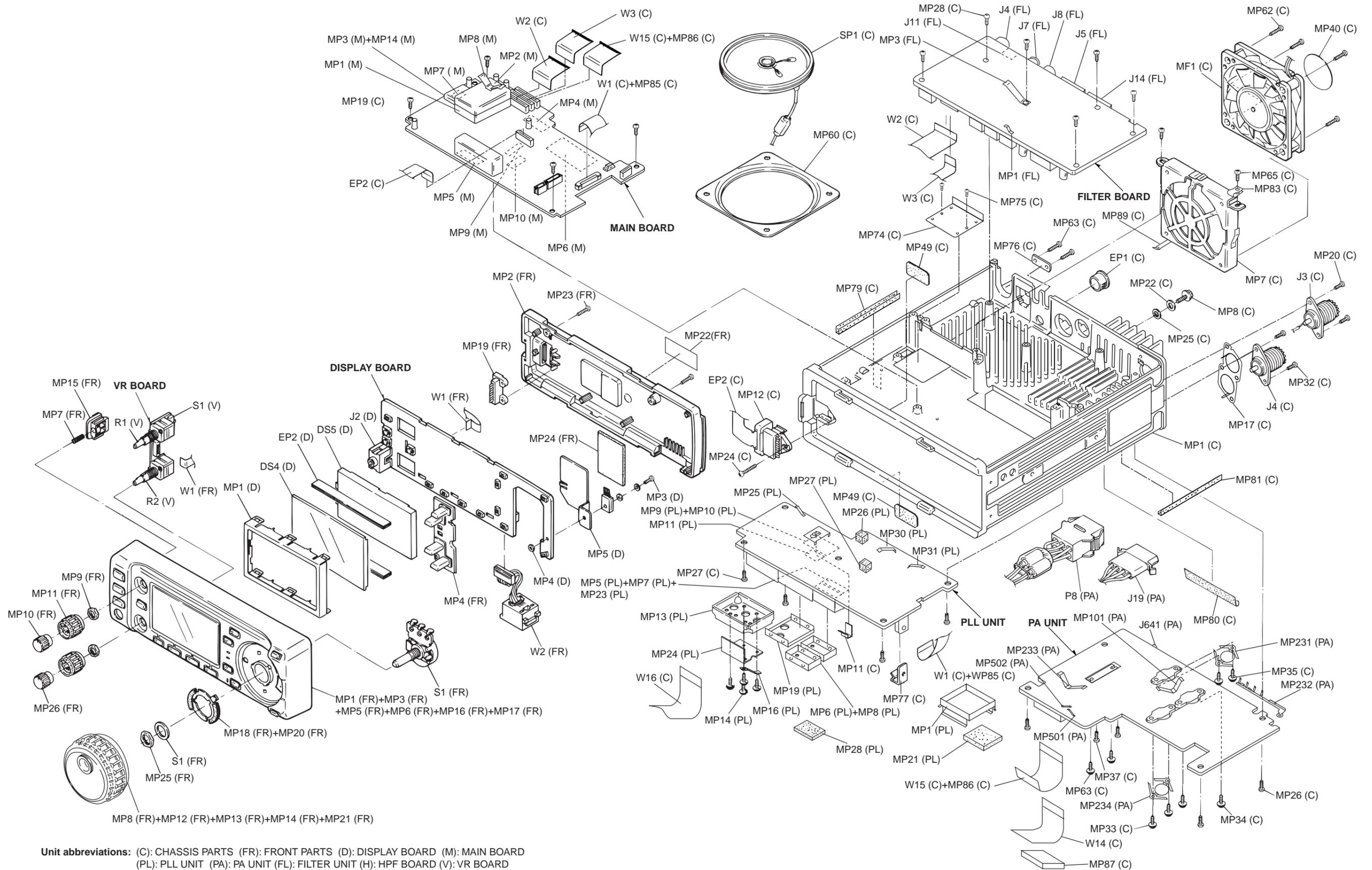
Unit abbreviations: (C): CHASSIS PARTS (FR): FRONT PARTS (D): DISPLAY BOARD (M): MAIN BOARD (PL): PLL UNIT (PA): PA UNIT (FL): FILTER UNIT (H): HPF BOARD (V): VR BOARD
