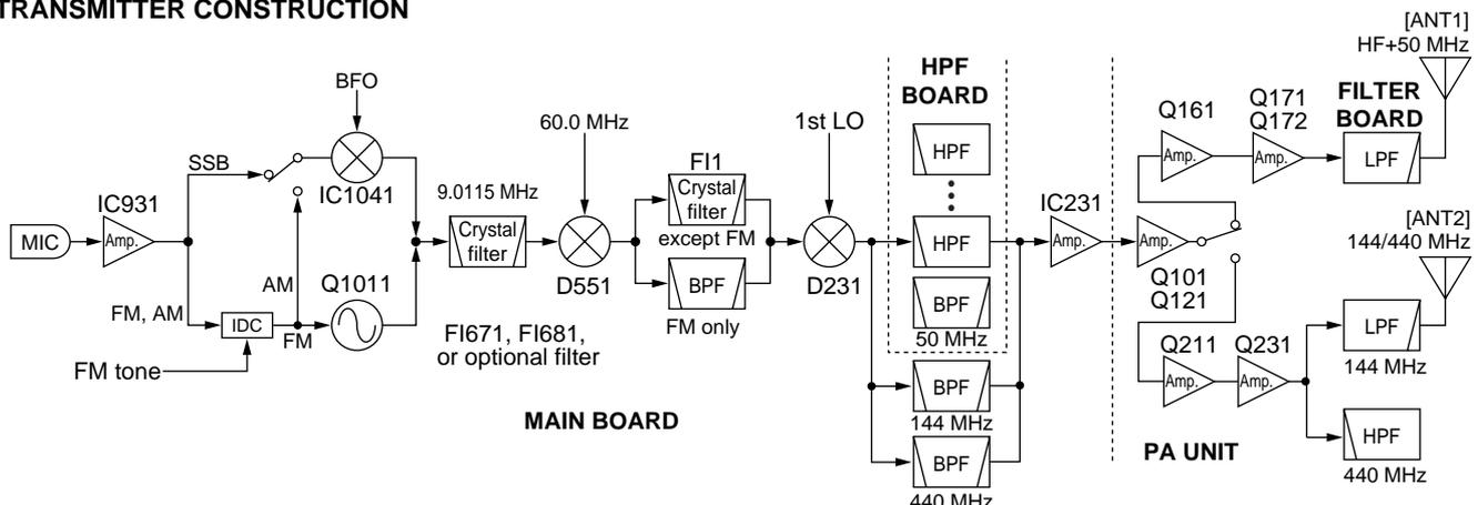
The 144 MHz RF signals from the 1st mixer (D271) via the low-pass filter (L251–253, C253–259) bypass the filters and pass through the bandpass filter (L182–L184, L195, L196, C181–C186, C195–C197) in the MAIN board. The signals are amplified at the RF amplifier (IC221) and YGR amplifier (IC231) and are then applied to the PA unit.
