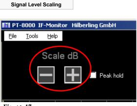
For scaling the signal level click the buttons and + below Scale dB top left of the program window.
