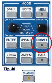
Recalling of VFO adjustments (frequency, mode and filter bandwidth) is done pushing the CHANNEL button located in the cluster MODE. It gives access to 3 banks of memory each storing 99 channels provided by PT-8000A.
