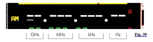
In this case the 1 Hz digit is not available for numerical input.
