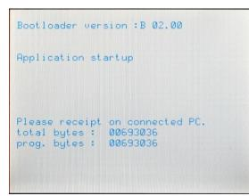
When data transfer is complete, on the display of the PT-8000A the message *Application startup* will point out the automatic restart of the transceiver after a short waiting period.
