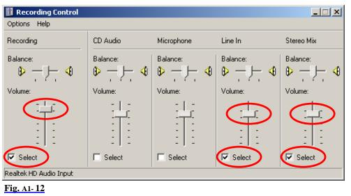
Make sure that sliders for Recording, Line In and Stereo Mix are located in upper position and the allocated Select boxes are checked.
