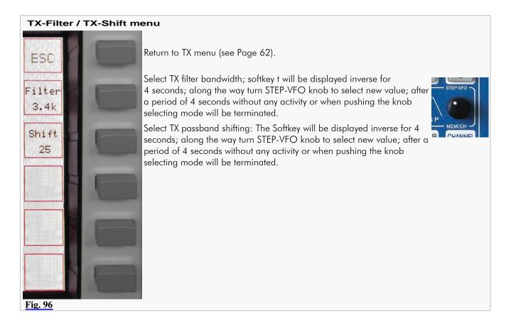
Turning STEP-VFO/MEM/CH knob will allow the following:
