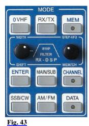
Pushing <u>MEM</u> button located in the cluster MODE will store the frequency and additional VFO values of the *active* RX to one of the 297 memory channels organized in three banks with 99 memory channels each bank.
