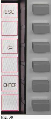
Numerical input will be aborted; the last used frequency will be displayed instead; the last used softkey menu will be called up.
