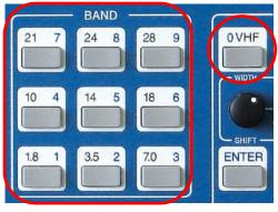
Pushing a band pushbutton selects one of two stored frequencies within the desired band (see Table 13 and 14).
