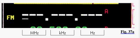
The number of blanks/diaits are shown depends on the resolution selected by using the Softkeys STEP  $\checkmark$ , STEP  $\checkmark$  or STEP VFO (s. P. 41). E.g. the resolution is 1 kHz the frequency will be displayed as follows:
