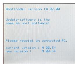
In case the new operation program has the same version number as the current version on PT-8000A, the display will show a warning notice and in the lower area these (identical) numbers.
