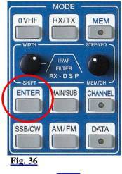
Pushing <u>ENTER</u> button located in the cluster MODE will call up the ENTER menu and will activate the numerical frequency input:
