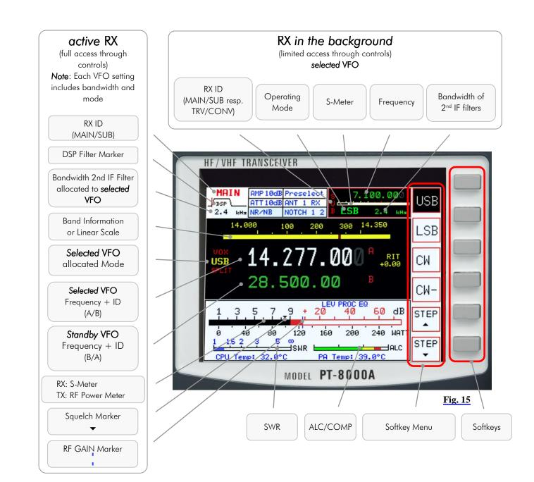
Softkeys and Softkey Menu The six keys (so-called *softkeys*) right next to the display give access to the functions named on the display at right border (in the *Softkey Menu*). The functions can be: Activate a device function, selection of an adjustment option, call up of superior or submenu.
