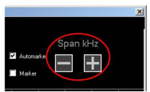
For scaling the panorama width click the buttons  $\square$  and + below Span kHz top right of the program window.
