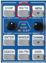
Pushing the button  $\overline{RX/TX}$  located in the cluster MODE will call up two types of menus which gives access to various basic settings for RX and TX.
