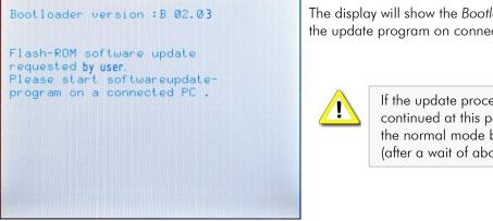
The display will show the Bootloader screen with a prompt to start the update program on connected PC.
