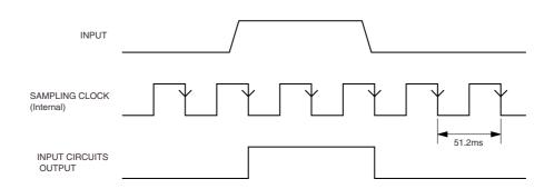
Note that data is read in on the falling edge of the sampling clock.
