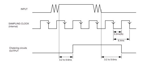
Note that the input is recognized during the LOW-level pulse interval,  $t_{\rm S}$  (32 ms), of the sampling clock.
