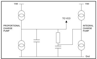
Fig.5 Loop filter using both charge pumps
