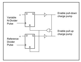
Fig.3 Auxiliary phase detector
