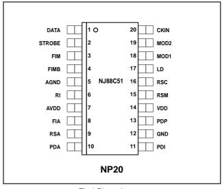
Fig.1 Pin assignment
