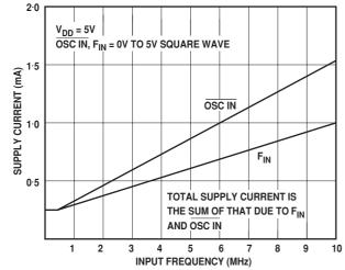
Fig. 3 Typical supply current v. input frequency
