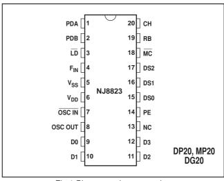
Fig.1 Pin connections - top view
