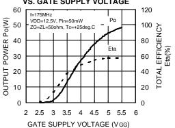
**TYPICAL PERFORMANCE** ( $T_{case}$ =+25°C,  $Z_G$ = $Z_L$ =50 $\Omega$ , unless otherwise specified)
