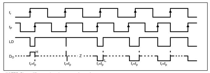
**NOTES:** Phase difference detection range:  $-2\pi$  to  $+2\pi$  Spike appearance depends on charge pump characteristics. Also, the spike is output in order to diminish dead band. When  $f_r > f_p$  or  $f_r < f_p$ , spike might not appear depending upon charge pump characteristics.
