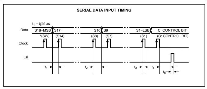
**NOTES:** Parenthesis data is used for setting divide ratio of programmable reference divider. On rising edge of clock shifts one bit of data in the shift register.
