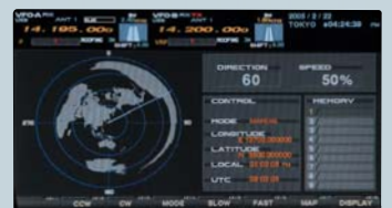
•Antenna Bearing Indication using Great Circle Map
