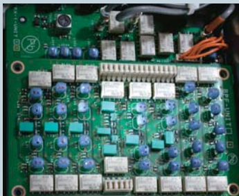
Bandpass Filter Unit (Amateur Radio band)
