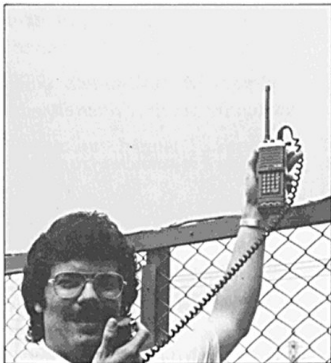
When using the YM-24 Speaker/Microphone, you can raise your FT-207R above obstacles that might ruin reception.
