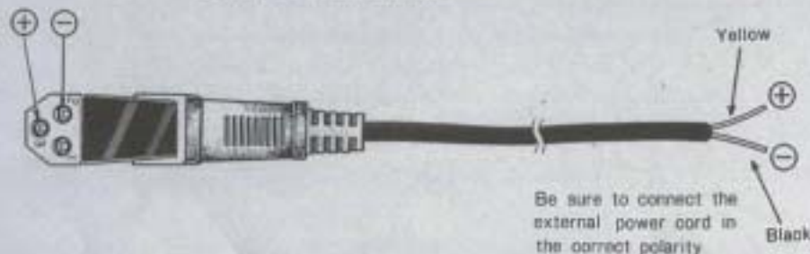
Fig. 7 Polarity of External Power Cord
